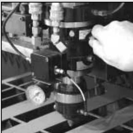
Lens removal is quick and easy with our lens cartridge system
