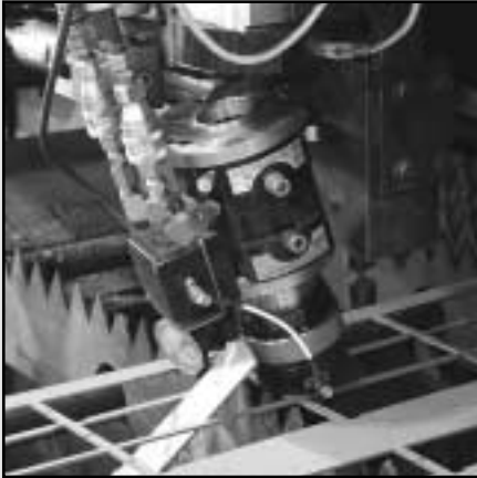
Crash occurs separating cutting head from machine
