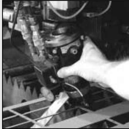
Operator resets head instantly with minimal downtime
