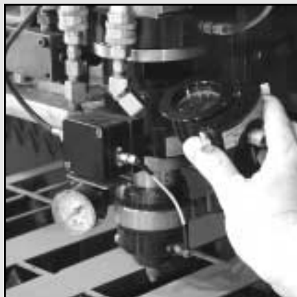
Simply slide the cartridge out to inspect, clean or change the lens
